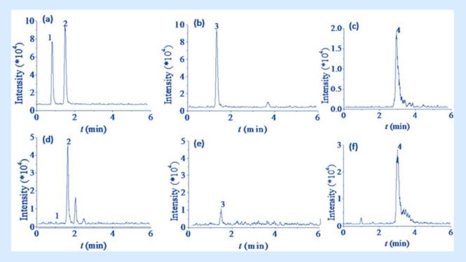
Figure 2: Extracted ion chromatograms of standard substances (a-c) and cannabis samples (d-f) by QDa confirmation analysis. Peaks: 1, CBD (m/z 315, ESI<sup>+</sup>); 2, CBN (m/z 311, ESI<sup>+</sup>); 3, THC (m/z 315, ESI<sup>+</sup>); 4, THCA-A (m/z 357, ESI<sup>-</sup>)
